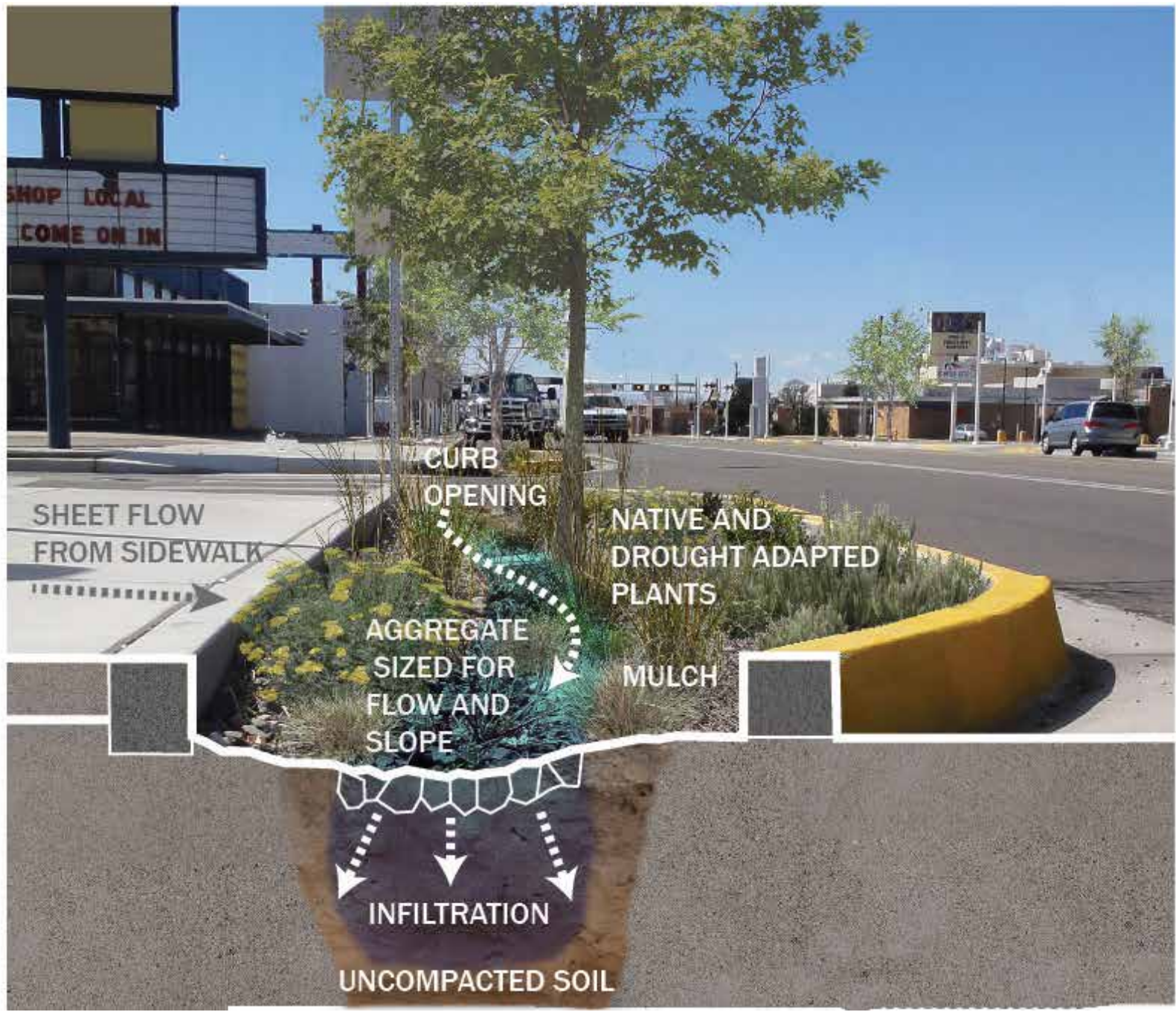
Stormwater Bumpout with Infiltration Conveyance
