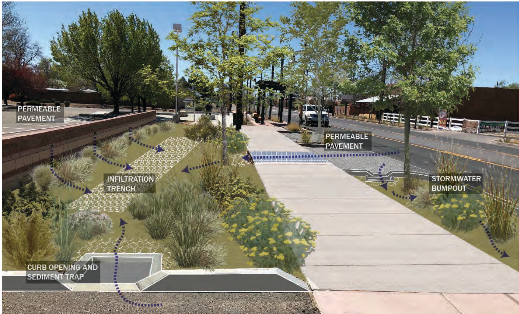
Example of a GSI/LID BMP Treatment Train with Permeable Pavement, Curb Opening with Sediment Trap, Stormwater Bumpout, and Infiltration Trench
